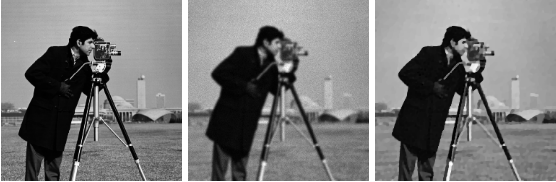
Figure 2: Left: Original 'cameraman' image of size 256 \times 256 . Middle: Image blurred by a Gaussian kernel (standard deviation \sigma = 1.3 ) and contaminated by Poisson noise ( I_{\max} = 1000 ). Right: Deblurred image by model (3) with \lambda = 0.01 .
